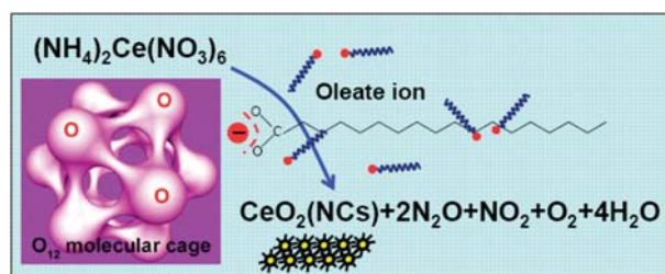
Fig. 3 Schemes of the icosahedral structure of Ce(NO 3 ) 6 2- and the synthesis process (for details see ESI†).
